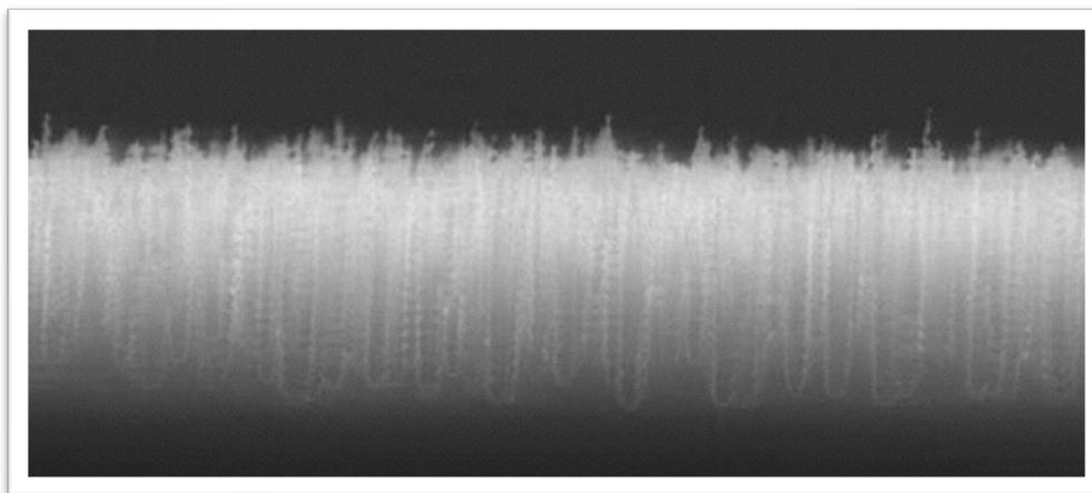
**Figure 1:** *Nanomolecular SiO<sub>2</sub> crystalline-like structures visualized under high powered electron microscopy. Once dried onto a treated surface, the structures covalently bond to the underlying base substrate, creating a newly modified, antimicrobial, protective surface barrier.*
